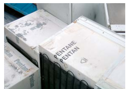
Even CFC-free refrigerators must be specially treated.
